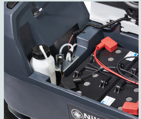
Detergent mixing system gives the user the option to clean with water only and to add detergent when really needed
