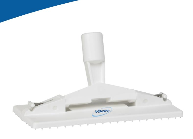
An excellent tool for cleaning walls and tanks. Often used to scrub stubborn dirt e.g. pastry, meat, sticky glucose type ingredients. The swivel neck allows the operator to clean underneath equipment. It is designed to hold a scouring pad of varying roughness. The clip mechanism is stainless steel and is very robust. This mechanism prevents the pad from falling off once heavy with water.
