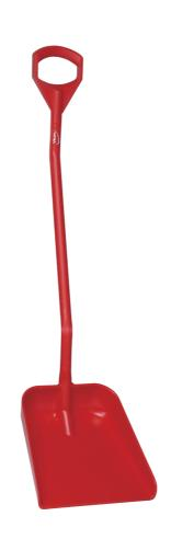
Robust hygiene shovel. The handle of this shovel is re-inforced with an inner aluminium tube. It is stepped in two places which helps to prevent back injuries. The neck joint has been strengthened in order to withstand heavy duty use. The short handle and small blade combination make it light weight and able to fit into smallish containers. Sometimes use as a large-scale dustpan.
