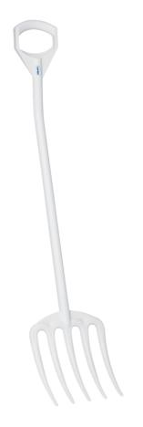
The hygiene fork is mostly used to empty out fresh produce from large containers, e.g. during grape harvest for wine making. The handle is re-inforced with an inner aluminium tube. It is stepped in two places which helps to prevent back injuries. The neck joint has been strengthened in order to withstand heavy duty use.
