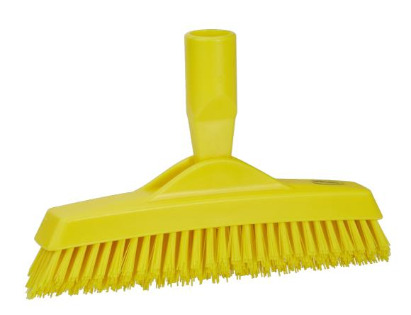
The crevice scrub is suitable for cleaning difficult to reach areas under and between equipment since the handle can be positioned parallel to the floor. The filaments are placed in an arrow shape that ensures are very efficient cleaning of even small cracks and crevices. The middle row of filaments are stiffer than the other filaments to form a very stiff scrubbing brush.
