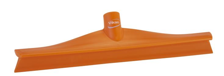
This ultra hygienic squeegee has a very soft and effective rubber lip, which ensures effective cleaning of floors and other surfaces. The rubber lip is angled to facilitate cleaning close to walls and around equipment without any problems. The squeegee's splash guard ensures that the liquid is not splashed onto the dried surface.
