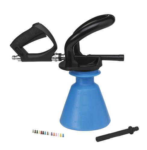
Cleaning in sanitary and small processing areas. Foam is applied with the foam sprayer without aerosols at normal water pressure. Always correct dosage ratio at 0.4-10%. Identification of chemicals facilitated by the colour-coding of the container. Use Safeone, 9340 as protection against chemical reflux in potable water supplies. Approved according to EN 1717 - substance class 3.
