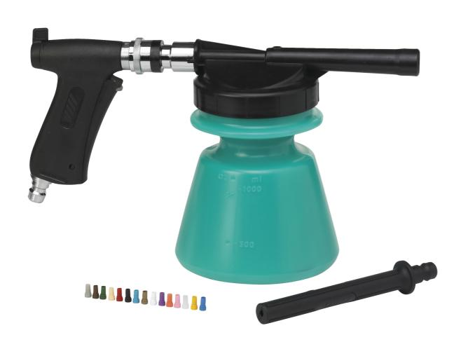
Cleaning in sanitary and small processing areas. Foam is applied with the foam sprayer without aerosols at normal water pressure. Always correct dosage ratio at 0.4-10%. Identification of chemicals facilitated by the colour-coding of the container. Use Safeone, 9340 as protection against chemical reflux in potable water supplies. Approved according to EN 1717 - substance class 3.
