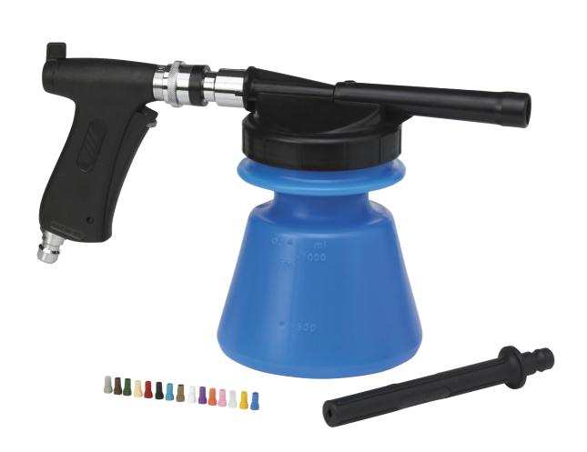
Cleaning in sanitary and small processing areas. Foam is applied with the foam sprayer without aerosols at normal water pressure. Always correct dosage ratio at 0.4-10%. Identification of chemicals facilitated by the colour-coding of the container. Use Safeone, 9340 as protection against chemical reflux in potable water supplies. Approved according to EN 1717 - substance class 3.
