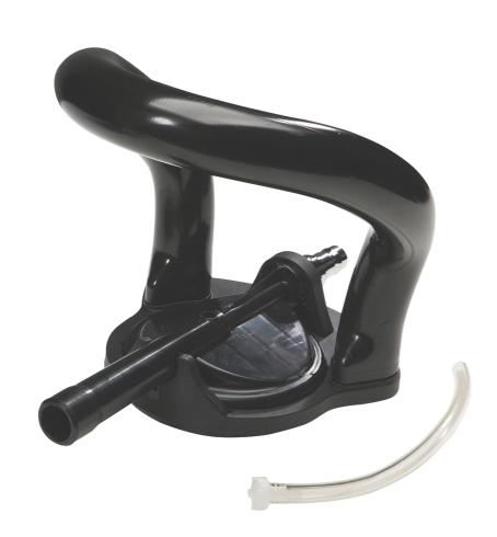
Ergonomic and solid handle with foam injector for foam cleaning. Water and chemicals are always mixed in correct dosage ratio 0.15 - 10% and are foamed on the surfaces. Fit both large and small container. Suction hose and filter provided.
