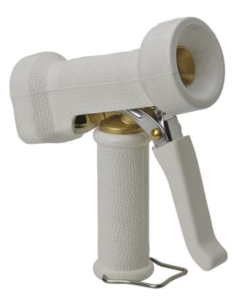
Suitable for cleaning floors and machinery including rinsing off work surfaces and walls after chemical foaming. Squeezing the rubber isulated trigger determines the jet pattern. The water jet can also be adjusted using the screw at the end of gun. The arrow on the gun shows the water spray direction. Use 0712, 1/2" or 0715, 3/4" hose nipples to be screwed into the bottom of the gun.
