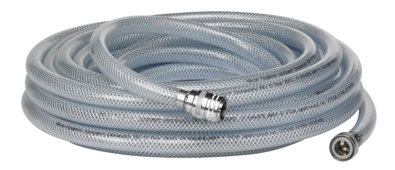
For cleaning where cold water is used at a maximum of 40° C. 0.5 inch hose ready for use. 0.5 inch clutch housing connected in both ends of the hose. Nipple for water tap provided for 0.5 inch, 0.75 inch and M22x1 screw thread types.
