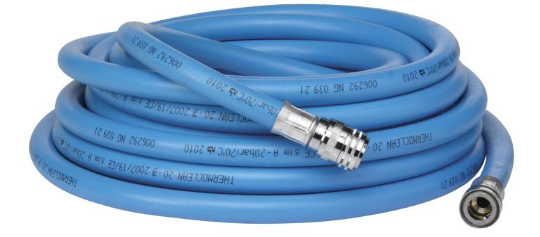
For cleaning where water is used at a maximum of  $70^{\circ}$  C. 1/2" clutch housing connected in both ends of the hose. Nipple for water tap provided for 1/2" inch, 3/4" and M22x1 screw thread types.
