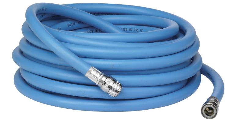
For cleaning where water is used at a maximum of  $70^{\circ}$  C. 1/2" clutch housing connected in both ends of the hose. Nipple for water tap provided for 1/2" inch, 3/4" and M22x1 screw thread types.
