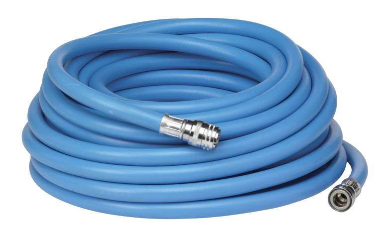
For cleaning where water is used at a maximum of 70° C. 1/2" clutch housing connected in both ends of the hose. Nipple for water tap provided for 1/2" inch, 3/4" and M22x1 screw thread types.
